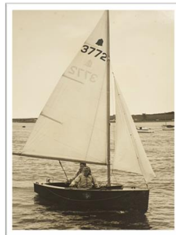
1960-nb wooden mast & boom, jib with hanks, lifting handles on fore and aft deck. Early attempt at centre sheeting. Lucas sails.
